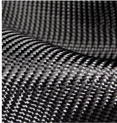
**Materials:** Featuring advanced thermally stable carbon-composite airframes, XB-1 and Overture are easier to fabricate and lighter than aluminum, maximizing fuel efficiency.
